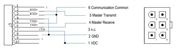
When setting the reader for MDB protocol (see 4.3.4 Dip-SwitchSettings), the 10 poutputs must be converted to the 6p MDB standard cable from the master pcb of the machine. Adapter cable is available (ref. S-031005-000).
