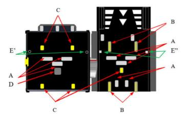
5. Check that the two sensor pairs S' and S" matching the stacker and the banknote (two pairs on the stacker back and two on the inner side of the case are clean (see section 5.1: Sequence of 2 blue blinks). PAY ATTENTION: do not use organic detergents (ex. alcohol, thinners, or petrol). Use only isopropyl alcohol.
