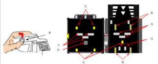
A. Optic sensors B. Traction Rollers C. Matching wheels D. Magnetic Sensor (only in LB-MU02, LB-LU11, LB-MU12)
