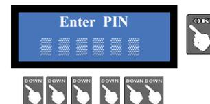
The display will now ask to confirm the entered 6-digit code; insert it again: the initialization of the ACS Cashless reader will then be started. At the end, the display will confirm that the ACS reader is ready, and will return to the configuration menu.
