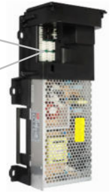
HUB PCB FOR CONNECTION OF THE PERIPHERAL UNITS
