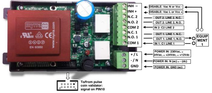
Service line 1(Pushbutton A): from pin 1 (COM 1) of the J2 connector, take a wire to the actuator of service line 1. If operation mode is "normally open", take the switching wire to the 1 actuator from pin 2 (N.O. 1). If operation mode must be "normally closed", take such wire from pin 3 (N.C. 1).
