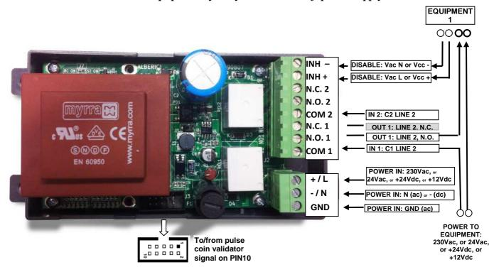
Service line 1 (Pushbutton A): from power supply, connect one end of service line 1 straight to the relevant actuator (i.e. electrical motor, solenoid, a.s.o.). Connect the other end to pin 1 (COM 1) of J2 connector.
