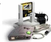
B2- Connect the USB cable between the PC and the USB-A slot on the slant side of the programmer box, *or else* connect the RS232 cable between the PC and the socket located on the slant side of the programmer box.
