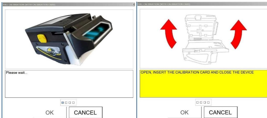
Once positioned the Calibration Card, press OK button and wait until confirmation of process ended.
