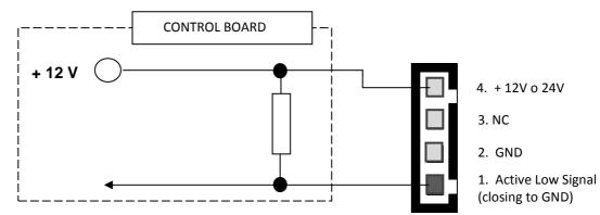
To make use of the ACS reader as replacement to a mechanical coin acceptor, whose switch simply provides a short-circuit when a coin is accepted, it is necessary to interpose a relay as shown below:
